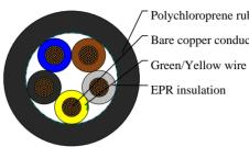
Polychloroprene rubber outer jacket Bare copper conductor
